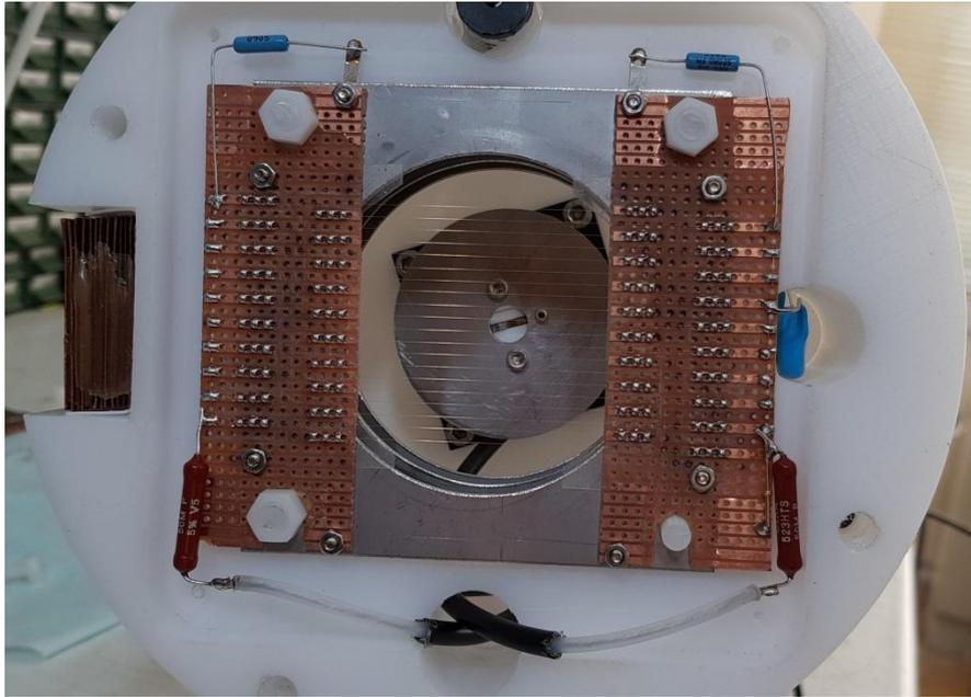
Fig. 1: Double grid cathode.
