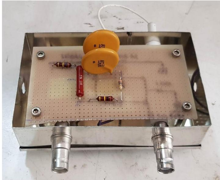
Fig. 6: High voltage pulse generator.
