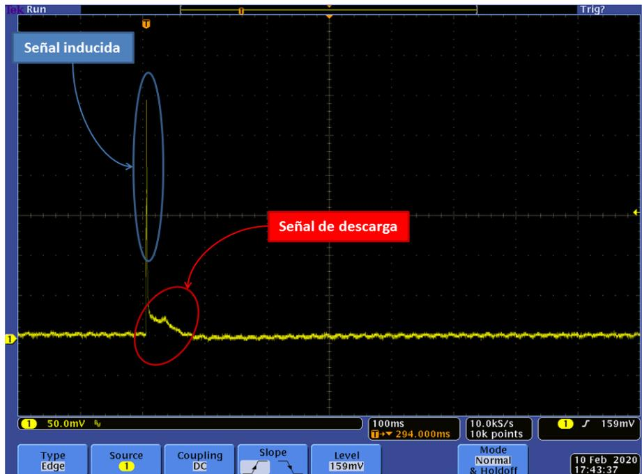
Fig. 4: Signal registered with the cathode at 0 V. The drift signal disappears and a discharge is visible.
