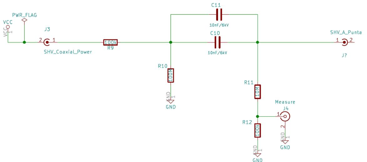
Fig. 5: Pulse generator circuit diagram.
