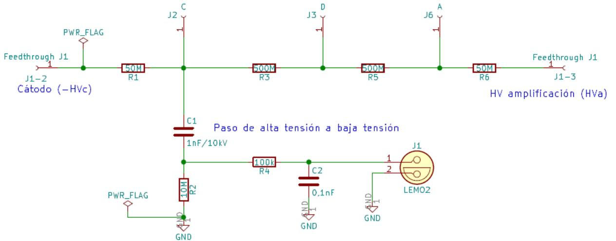
Fig. 2: Diagram of the cathode and the reading system.
