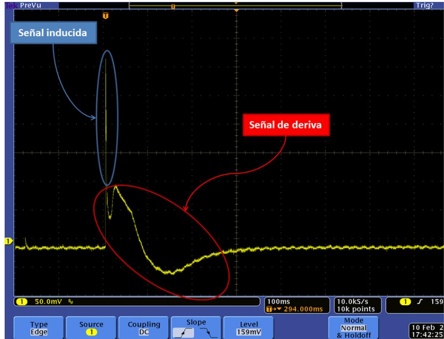
Fig. 3: Induction and drift signals produced at the needle and the cathode.
